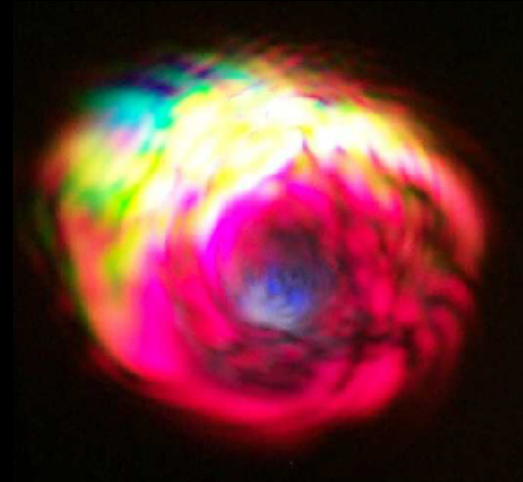
Plasma confined by liquid: \sim 5000\text{K} , \sim 10\text{GPa}
