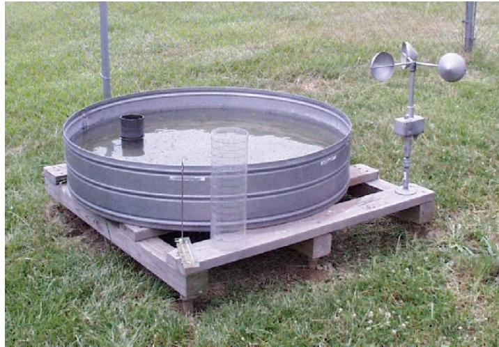
Evaporation pan. These are at some weather stations. Typically automated.
