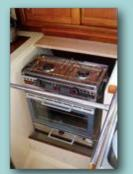
We upgraded to an Origo non-pressurized alcohol stove. No pipes, hoses, pumping or explosion hazard. Works great!
