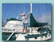
The new whisker pole track. Our "J" is 14.5 feet, but the pole can stretch to 22 feet so we can point higher with the pole pushed to weather.
