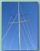
The new running backstays, made from T-900 with thimbles eye-spliced at the tangs. We will tension them with the weather sheet winch.
