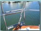
The new backstay, turnbuckle and Hi-Mod terminal. Now, there are just seven more wires to go, all will be 316 SS 9/32" (up from 1/4").
