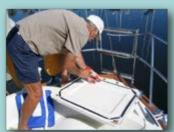
Attaching and cementing a new seal for the engine hatch cover.
