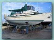
After the power wash, which removed most of the loose paint. The boat was then skirted and the rest was power sanded off.
