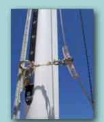
Detached stay is shackled to the mast such that it doesn't slap against the mast or kink. The plastic hose doesn't slip on the stay or shackle.
