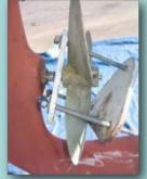
During our haulout, we pulled the prop. This was taken after we broke it loose with a prop puller along with a lot of heat from a propane torch.
