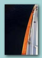
Using West System epoxy and filler, we repaired the ding. Now we need to sand and clean the rest of the caprail before varnishing. After three coats of Cetol Natural Teak. We will rub down and add a maintenance coat in six months. We did not apply a coat of Cetol Gloss, as some recommend, because we did not want the caprail to be too slick.
