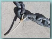
Chain markers that outlast the chain. By varying the lengths of the two tails, there are plenty of combinations to mark any chain. This is for 50
