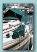
The pelican hook is attached at the beam cleat with the bagged sail still hanked on. It takes about three minutes to detach or reattach.
