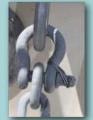
Properly moused Class 2 shackle. Tighten hand tight, then a 1/4 turn more by tool. Mouse so that pin cannot loosen. Tuck twist into hole.
