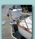
The Monitor is lashed to the stern with rope in order to steady it for measuring, leveling and bolting up.
