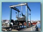
The lifting. This is the smaller of the two lifts at VHBY. They can handle up to 165 tons.
