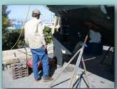
Removing the rudder in order to pull the propeller shaft.
