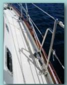
We acquired a small whisker pole so we can pole out the staysail. It greatly increases sail carrying options downwind.
