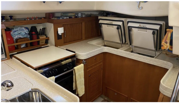
The mark of a superb galley: Double sinks, tall fiddles, massive top-opening refrigerators, a well-guarded gimbal oven. Yes, it's possible to prepare Christmas dinner for the whole anchorage. Courtesy of Yachtworld.com
