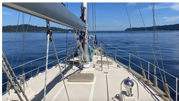
Principal sail controls including mid-boom sheeting lead aft to the cockpit. She's also fitted with mast pulpits, helping secure crew working forward. Note the side shrouds affixed to the exterior of the hull. Buyers should survey those terminals with care. Courtesy of Yachtworld.com
