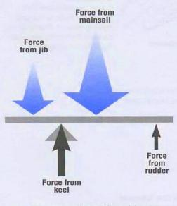
Forces on a sailboat act like weights on a see-saw (above), with the keel supporting the middle. If the force from one sail outweighs the other, the see-saw will tip (the boat will turn).
