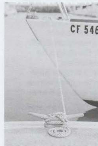
Cleated docking lines should always be secured with a cleat hitch
