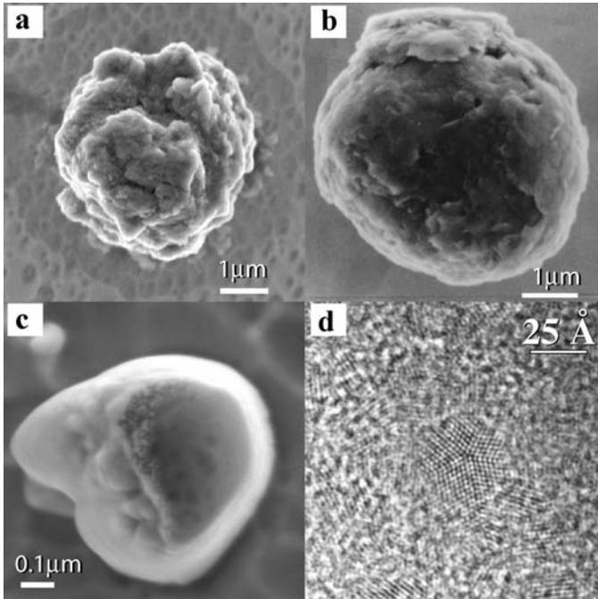
**Figure 1** (a) Scanning electron (SE) micrograph of 3  $\mu\text{m}$  presolar SiC grain (courtesy R. Stroud). (b) SE image of 5  $\mu\text{m}$  presolar graphite grain (courtesy S. Amari). (c) SE image of 0.5  $\mu\text{m}$  presolar  $\text{Al}_2\text{O}_3$  grain. (d) High-resolution transmission electron microscope image of presolar nanodiamonds (courtesy T. Daulton).
