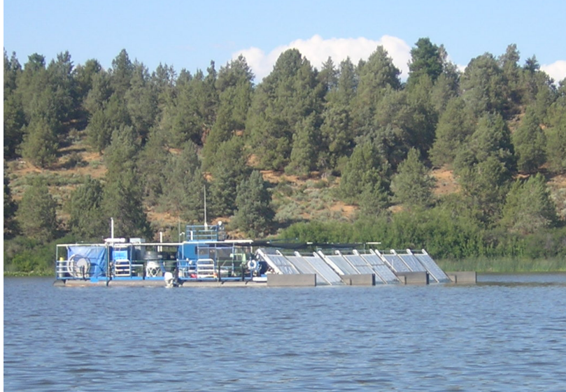
Figure 7. Harvester machine for skimming AFA off the surface of UKL. An obvious example that not everyone wants to have lower algal concentrations in the lake.
