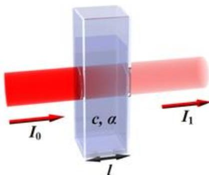
Figure 1- Absorption due to light passing through a medium
