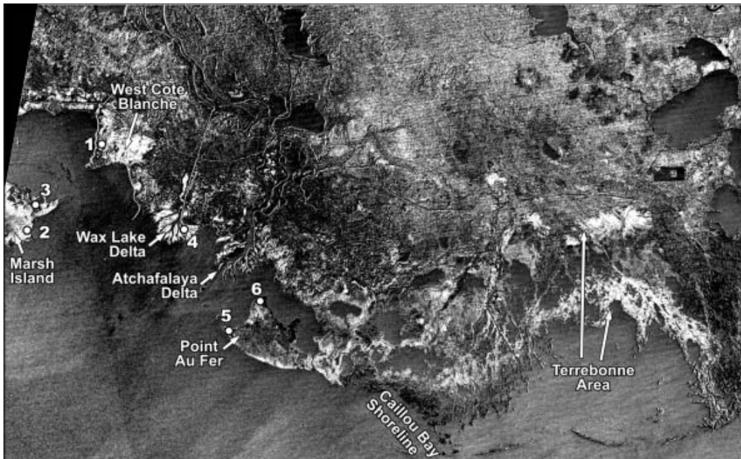
Figure 9: Difference image obtained by subtracting the mean DN values of 23 and 28 September 2002 SAR image from 3 October 2002 SAR Image (Lawrence et al. 2005)
