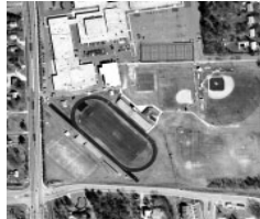
2.44-meter multispectral image Four bands: Blue, Green, Red, and Near-Infrared (click on image for larger version)
