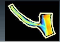
Project Setup Datum Conversion Convert LiDAR and Bathymetry to Point Data using Sample (Spatial Analyst) Delineate model study area by creating a water polygon using a conditional statement (from LiDAR) Buffer River polygon 200 feet, remove all LiDAR and bathymetry points from outside the buffer area.
