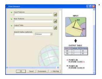
Both input and near features (layers) must have point geometry.
