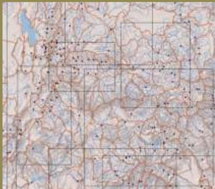
For a given USGS gauge station on a stream, determine the upstream extent of the contributing watershed
