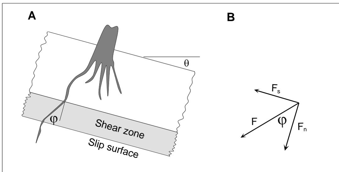
Figure 4. Role of tree roots in reinforcing a soil mass.
