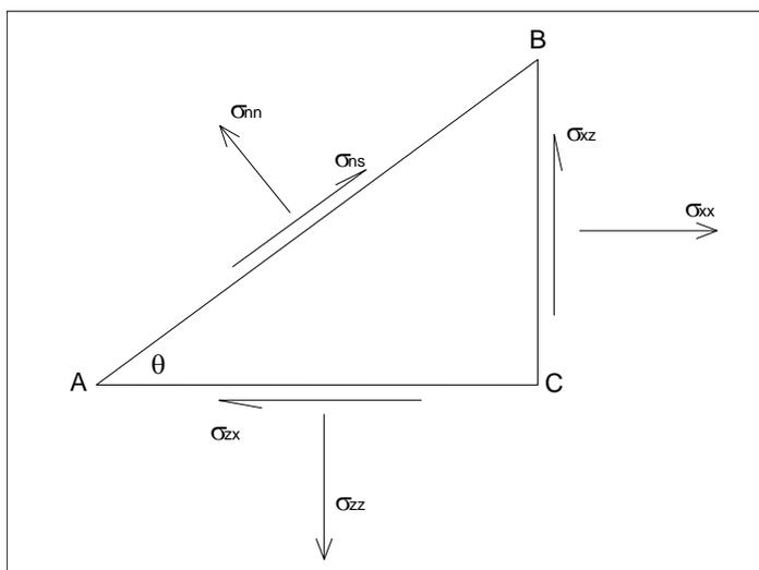
Figure 7. Definition diagram for (a) forces and (b) stresses.  $\sigma_{nn}$  is normal to some inclined plane,  $\sigma_{ns}$  are parallel to the inclined plane.
