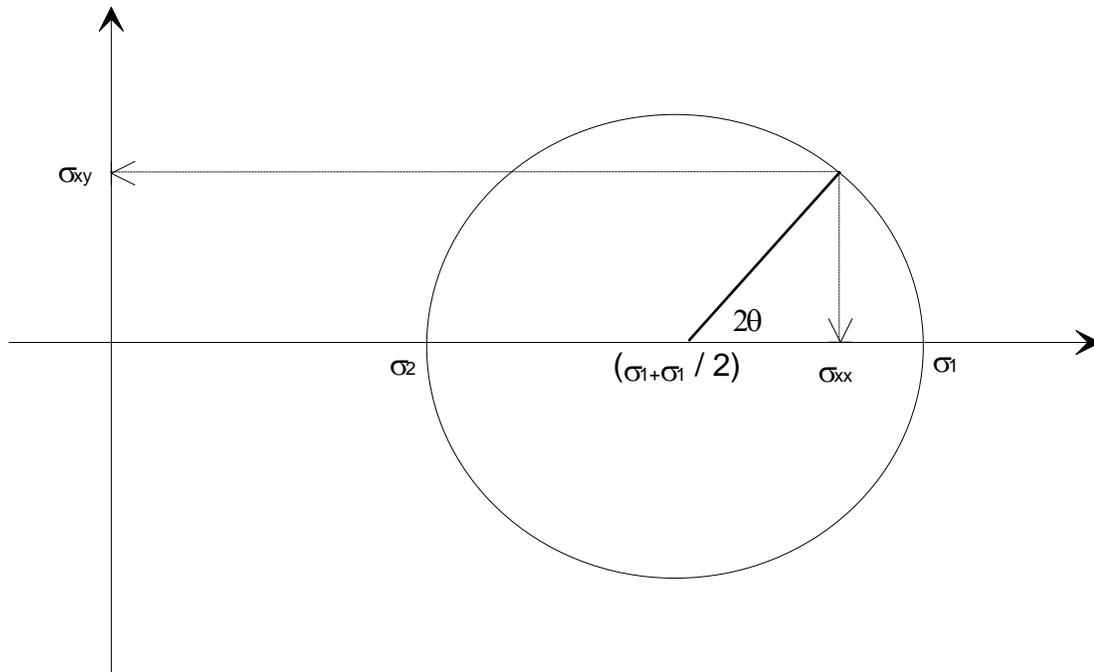
Figure 9. Mohr's circle showing the parameters in the equations derived above.
