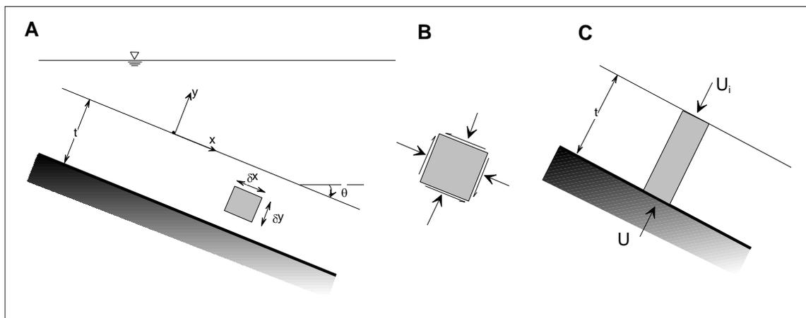
Figure 3. Definition diagram for a submerged infinite slope.
