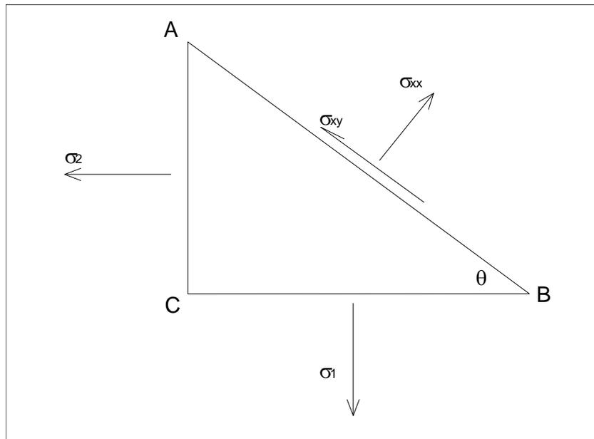
This is a very similar case to that considered above only in this case we know the principal stresses,  $\sigma_1$  and  $\sigma_2$ , so there are no shear stresses acting on those planes. We have defined a positive  $x$ - and  $y$ -coordinate system as shown in Figure 8. We assume that the body is in equilibrium, so we start by summing forces in the  $x$ -direction
