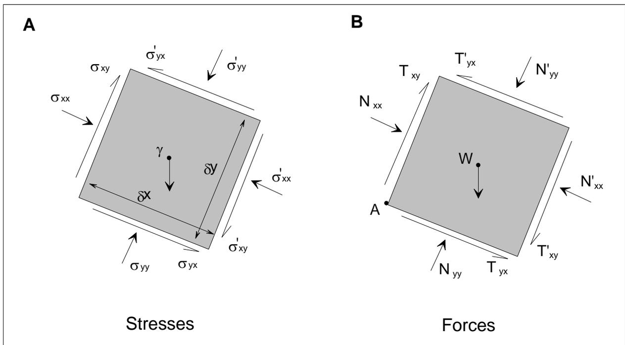
Figure 2. Unit element in a slide mass. Note that all the stresses shown are in their *positive* directions, so that normal stresses are positive if compressive.
