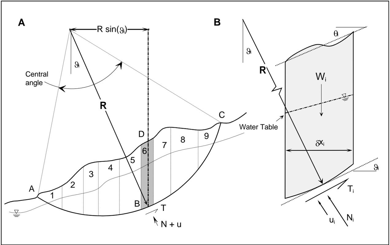
Figure 5. Definition diagram for Fellenius and Bishop methods. A simple slip surface is assumed, and the total moments are determined by summing moments for each slice. The factor of safety is defined as the ratio of the sum of the resisting moments divided by the sum of the driving moments.
