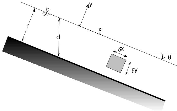
Figure 1. Definition diagram for infinite slope analysis
