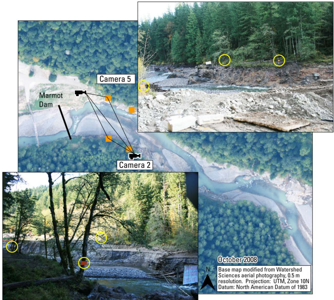
Figure 13. PhotoModeler creates a model based on coincident points between photographs. This example shows where rays from cameras 2 and 5 would intersect the orange photograph targets. Yellow circles indicate the location of targets within the terrestrial photographs.
