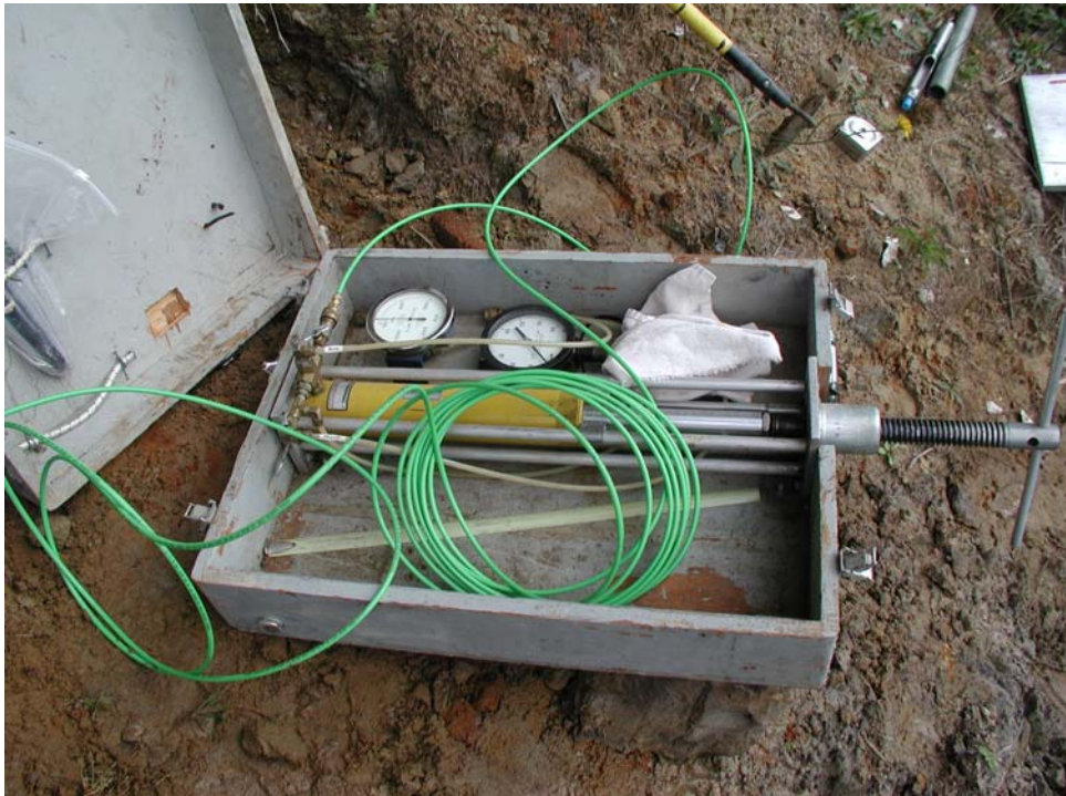
Figure 21: Photo of PuP pressuremeter control box and pressure gauges.
