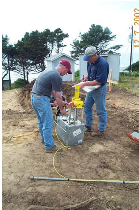
Figure 19: Photo of Texam pressuremeter control unit in use at the Ona 1A site located on the top of Ona Beach sea cliff.
