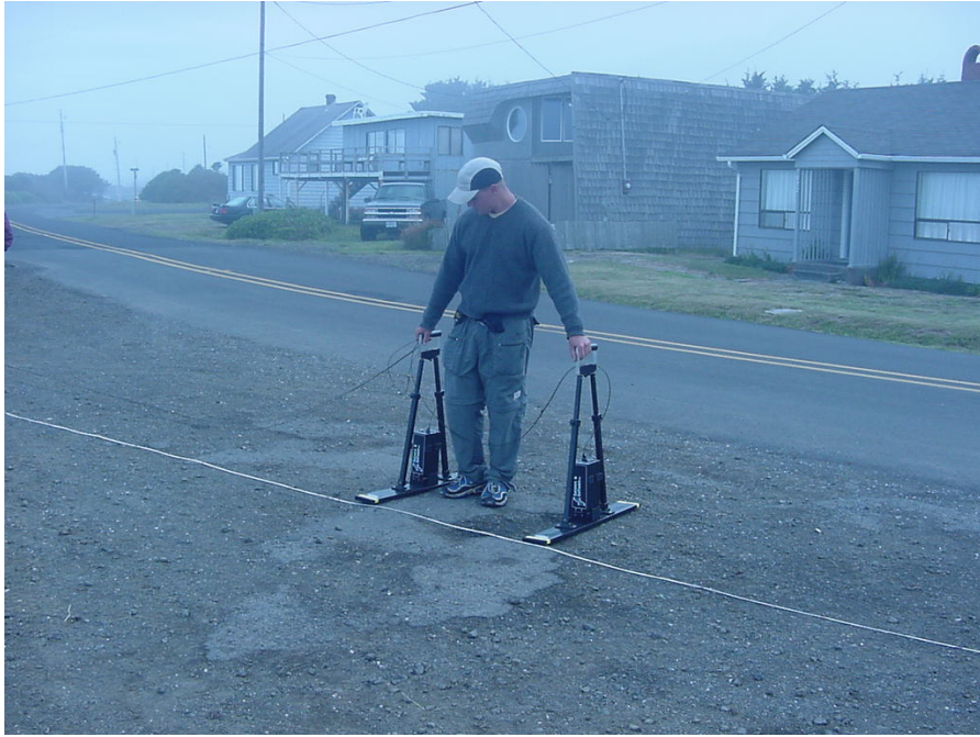
Figure 16: Photo showing GPR equipment with the 100 MHz antenna attached.
