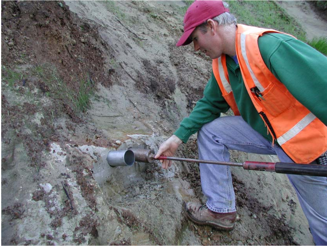
Figure 14: Photo showing soil sampling using a driven or pushed Shelby tube (on left in outcrop) and an AMS core sampler that holds six Dames and Moore brass rings (on the right).
