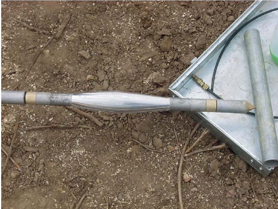
Figure 22: Photo of fully expanded EX pressuremeter membrane.
