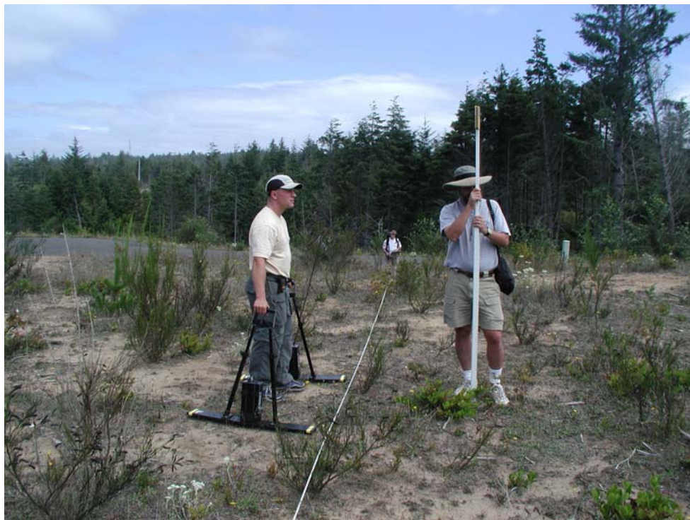
Figure 41: GPR profile line (facing east) at Pinecrest site using a 100 MHz antenna.
