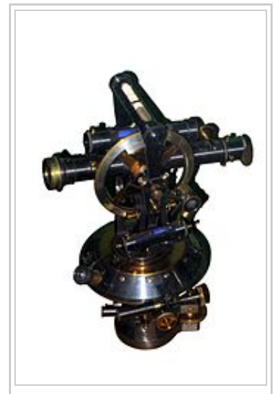
Sectioned theodolite showing the complexity of the optical paths
