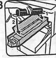
Fit the cartridge in the groove at the end of the black developer unit.
