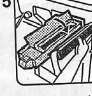
Put all the toner in the black developer unit. Carefully remove the cartridge.
