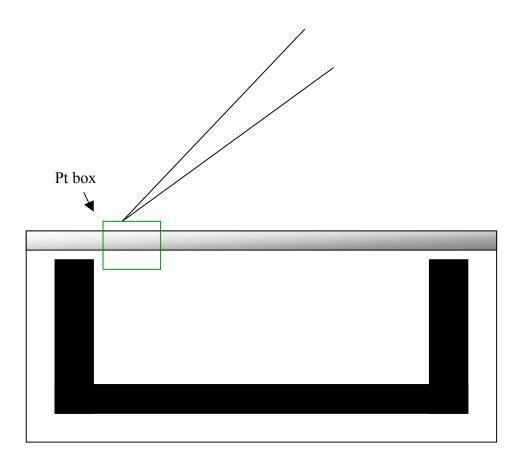
6. Cut the remaining "pt bridges" free with 100 - 500 pa, si.mtr, serial milling. LOWER the stage until the sample is out of the trench. Put the omniprobe in the parked location and retract the omniprobe and the pt gis.
