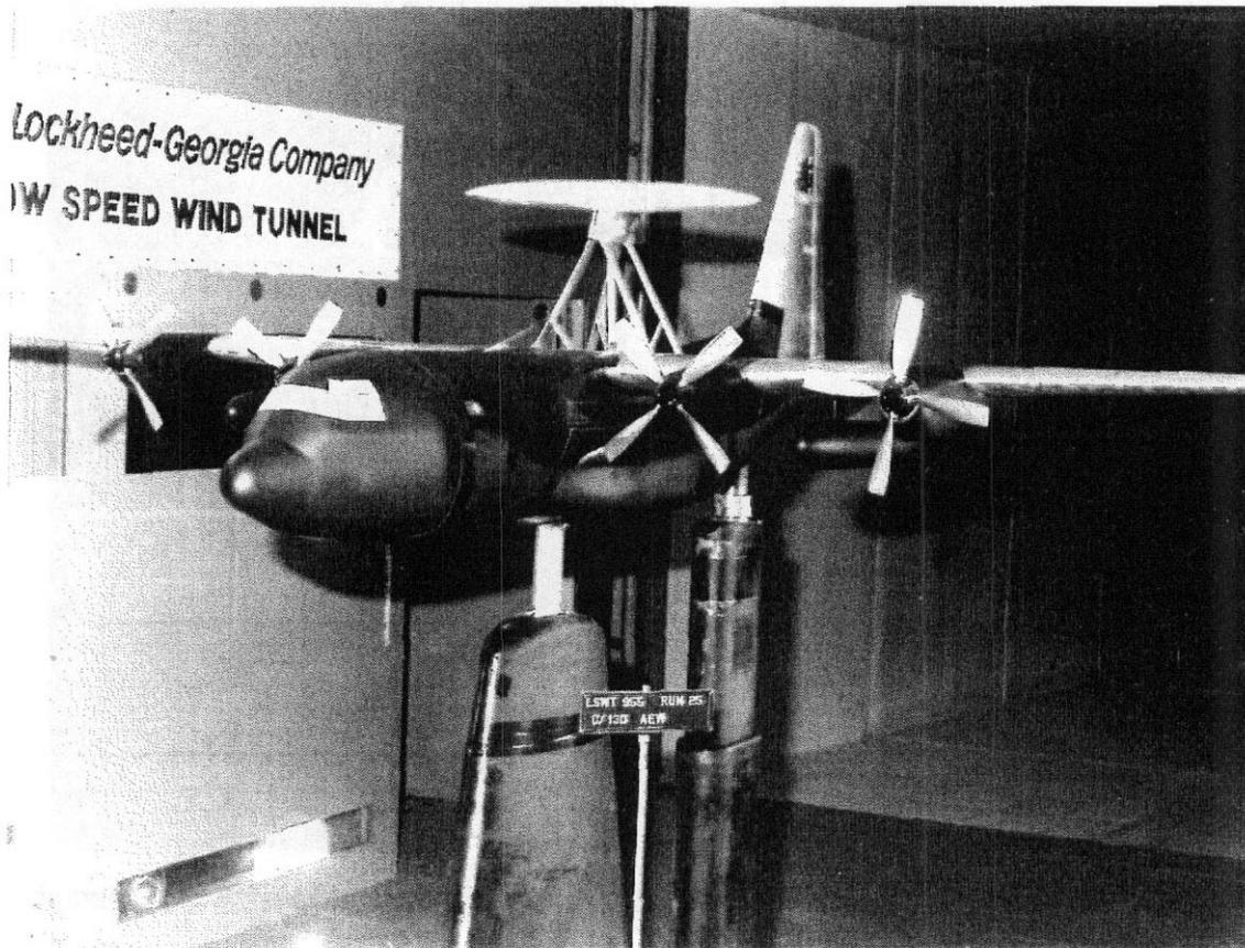
**FIGURE 737** Two-strut tandem. (Photograph courtesy of Texas A&M University Low Speed Wind Tunnel.)
