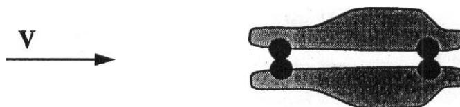
FIGURE 14.14 Symmetric models to obtain ground plane representation with no ground plane boundary layer.
