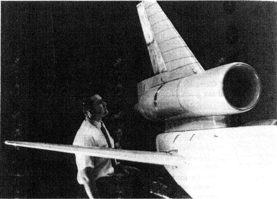
**FIGURE 18.6** DC-10 tail flutter model with double-hinged rudder. (Photograph courtesy of NASA Langley and McDonnell-Douglas Corporation.)
