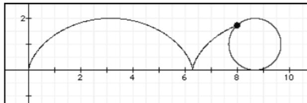
A cycloid has the parametric equation  $x = r(\theta - \sin\theta)$  and  $y = r(1 - \cos\theta)$  where  $r$  is the radius of the generating circle and  $\theta$  is the amount of rotation of the circle in radians.
