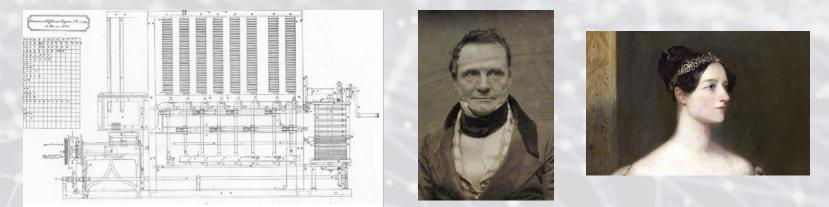
• Babbage later proposed (1837) the *Analytical Engine*, a general-purpose computer (never built due to inadequate funding) that incorporated an arithmetic logic unit, control flow (e.g. for loops) and integrated memory. Note that <u>the first physically-realized</u>, general-purpose computer did not appear <u>until over a century later</u>, in 1941, with the 'Z3' designed by Konrad Zuse.
