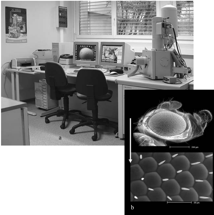
Figure 3.1. The environmental scanning electron microscope: a) a general view of the environmental scanning electron microscope, b) example: detailed makeup of the eye of a drosophila
