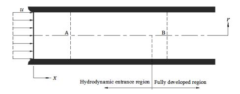
3. For a thermal boundary layer in a circular tube sketch the variation of the thermal boundary layer thickness  $\delta_t$  in the thermal entrance region. Sketch the temperature profiles in the entrance region (A) and the fully developed region (B) (3 pts).
