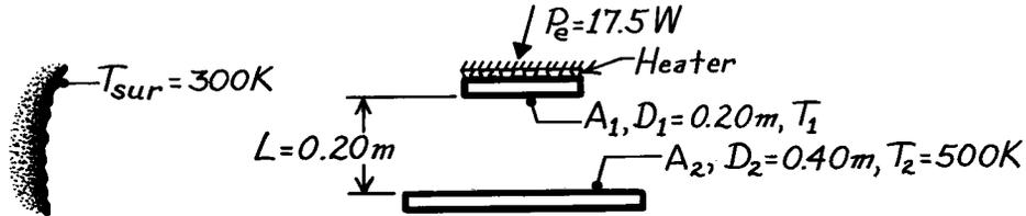
**ASSUMPTIONS:** (1) Plates are black surfaces of uniform temperature, and (2) Backside of heater on  $A_1$  insulated.
