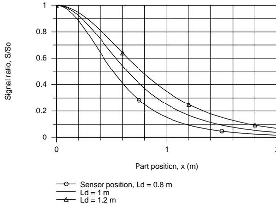
When the part is directly under the sensor,  $x = 0$ ,  $S/S_o = 1$  for all values of  $L_d$ . With increasing  $x$ ,  $S/S_o$  decreases most rapidly with the smallest  $L_d$ . From the IHT model we found the part position  $x$  corresponding to  $S/S_o = 0.75$  as follows.
