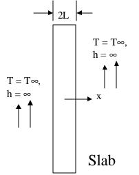
• Discretize the governing equation and boundary conditions for this problem by writing in explicit finite difference form for the time dependent temperature distribution T(x,t) in the slab.
