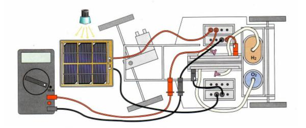
Example of a color diagram from the Fuel Cell Car & Experiment kit lab manual. The lab manual is needed for proper use of this companion curriculum.
