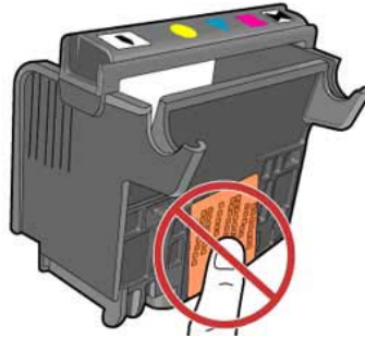
Figure 5: Do not touch the contact area with your finger
