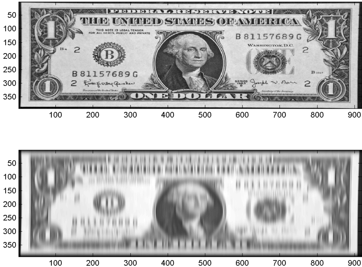
Figure 7. Image blurring through diffusion. Each pixel of the image has associated a value (typically from 0 to 255, or scaled to values between 0 and 1) that represents its gray scale intensity. High values are associated with "hot" (high density) regions whereas low values are associated with "cold" (low density) regions. The diffusion process applied to an image (top figure) transfers the gray scale intensity from high values to low values and produces a blurred image (bottom figure).
