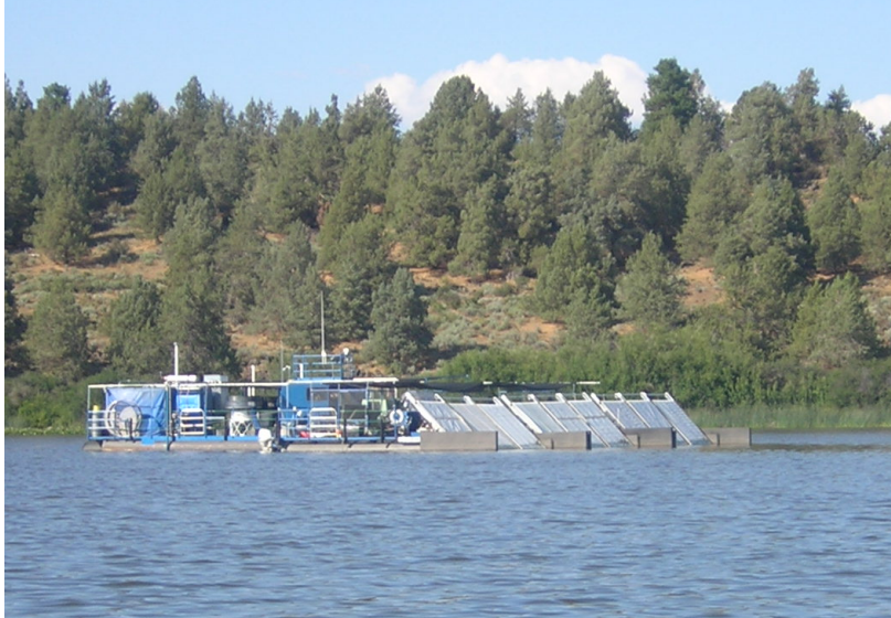
Figure app2-2. Harvester machine for skimming AFA off the surface of UKL. An obvious example that not everyone wants to have lower algal concentrations in the lake.
