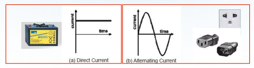
The grid electricity is Alternative Current (AC) Each wire changes from + to - 50 times or 60 times per second
