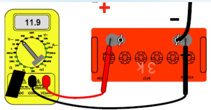
Warning! DO NOT try to measure a (short circuit) battery current like this, you would destroy the voltmeter!
