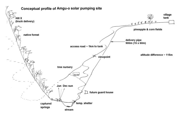
Due to rainy season damage to the access roads, truck delivery happened on the hill marked X (left of drawing), about 1km farther away than planned. Plus, there was a steep path to reach the site from the road.
