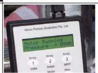
At 4pm, the pressure reaches about 100m and stops rising. The pump turns slowly, but apparently there is not enough sun to push the water all the way up the hill.
