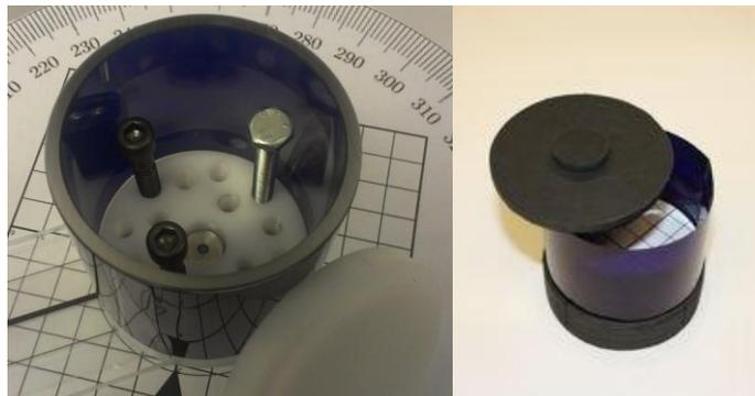
The enclosure was made with [Congo Blue #181](#) lighting filter with an acrylic base and lid. An earlier version of the enclosure was made with foam board. The light filter is attached to a clear plastic tube. It is important that the walls are thin and that they are transparent to the IR light of the photogate.
