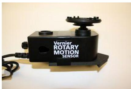
[Rotary Motion Sensor](#) We also made an angle indicator made of clear plastic. See the picture of the complete setup below. There are holes on either side of the plastic angle indicator that fit over the post of the rotating platform and the rod holding the rotary motion sensor, which is connected to the angle indicator with Velcro.
