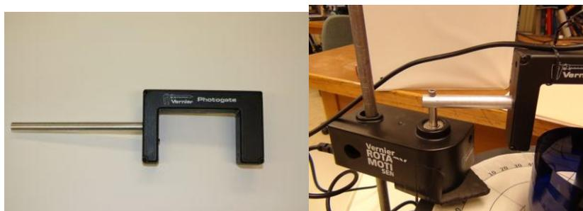
[Photogate sensor with extension rod](#) (included). NOTE: We have found that setup is greatly simplified by eliminating the clamp that holds the photogate rod to the rotary sensor and simply drilling a hole in the rod so that it can be screwed directly into the shaft of the rotary sensor.
