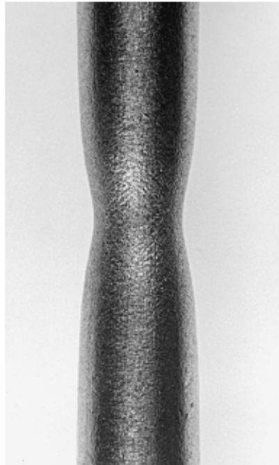
Figure 6-7 Neck down of a tensile test specimen within its gage length after extension beyond the tensile strength. (Courtesy of R. S. Wortman)
