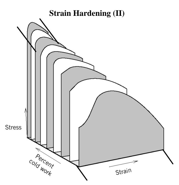
Yield strength and hardness are increasing as a result of strain hardening but **ductility is decreasing** (material becomes more brittle).
