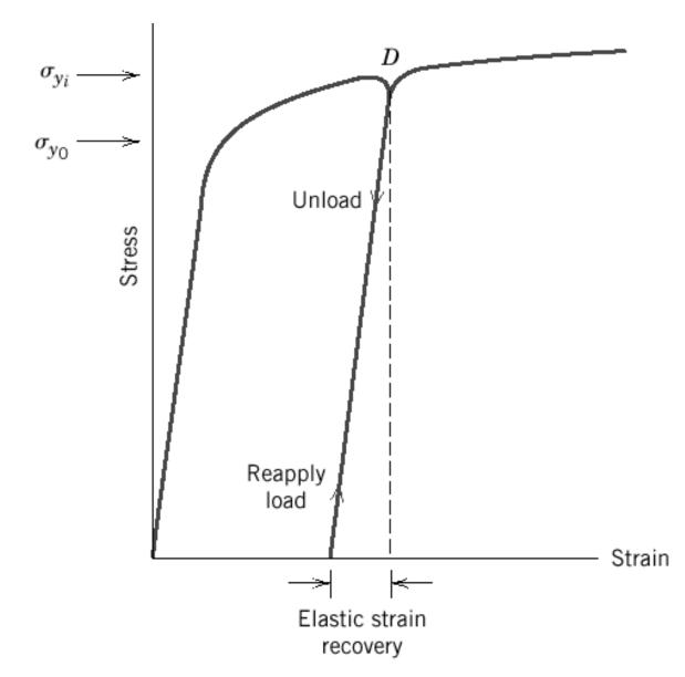
The new yield strength,  $\sigma_{yi}$ , is higher than the initial yield strength  $\sigma_{yo}$ . The reason for this effect - strain hardening.
