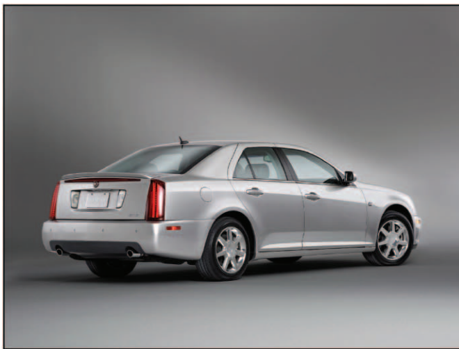
Figure 8. Quick plastic-forming (QPF) technology provides an intersection of art and science that can produce an "edgy" look that satisfies GM's designers. A good example is the trunk lid on the Cadillac STS. With QPF, the trunk lid can be fabricated in a single piece without sacrificing the clean, sharp edge.
