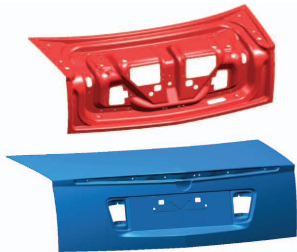
Figure 8. Quick plastic-forming (QPF) technology provides an intersection of art and science that can produce an "edgy" look that satisfies GM's designers. A good example is the trunk lid on the Cadillac STS. With QPF, the trunk lid can be fabricated in a single piece without sacrificing the clean, sharp edge.
