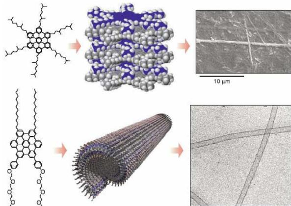
**Figure 9.** Examples of Molecular Self-Assemblies formed by hexabenzocoronenes: (left) molecular structure; (center) MSA simulation; (right) scanning and transmission electron microscope images of the respective MSAs. (From [25]. Reprinted with permission from AAAS, © 2004)
