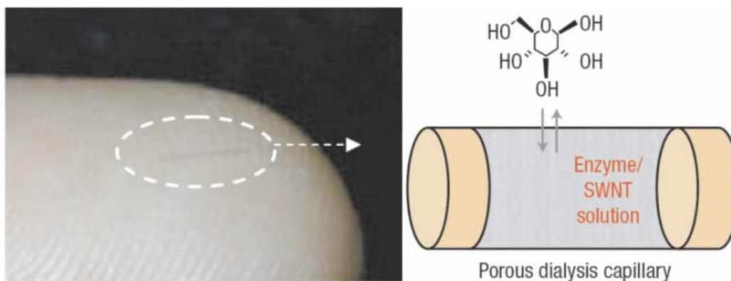
**Figure 7.** A permeable capillary, shown to size on a human finger, is loaded with the nanotube solution allowing glucose to diffuse through the membrane with the containment of the sensing medium. On placing the capillary beneath a human epidermal tissue sample, one can map the nanotube fluorescence from the capillary. (Adapted by permission from Macmillan Publishers Ltd: Nature Materials [21], © 2005)
