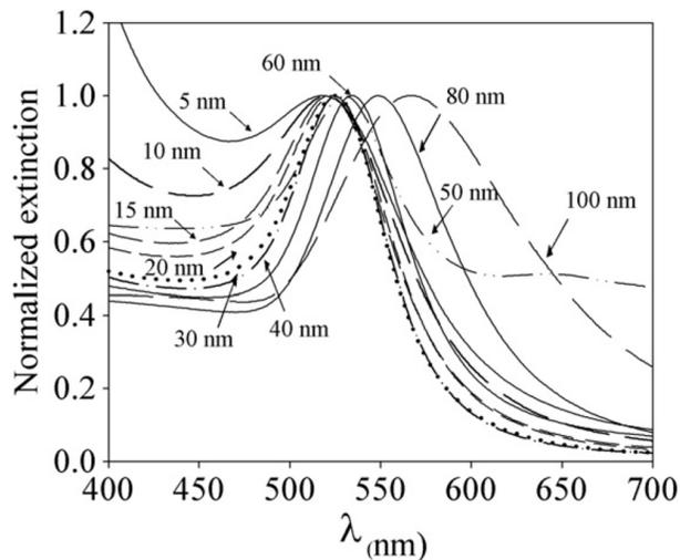
**Figure 3.** Extinction coefficient versus wavelength of gold colloidal nanoparticles in aqueous medium. The different spectra correspond to different sizes of the gold nanoparticles. (Reprinted by permission from IOP Publishing: Nanotechnology [9], © 2005. Courtesy of C. Rinaldi.)
