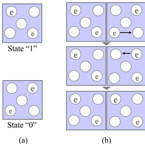
**Figure 10.** Quantum-Dot cell [27]. (a) Two states of equal energy in a Quantum-Dot cell. (b) Transfer of a “1” to the next cell. (See details in the text.)
