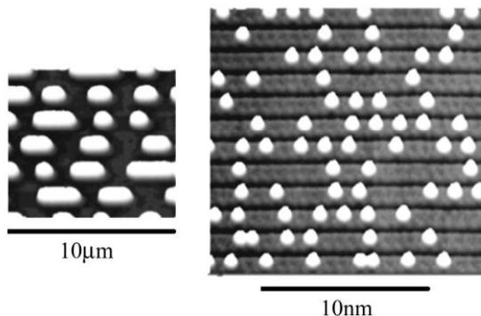
**Figure 2.** Comparison of the atomic memory on silicon (rhs) with a CD-ROM (lhs). (Reprinted by permission from IOP Publishing: Nanotechnology [4], © 2002. Courtesy of F. J. Himpsel.)
