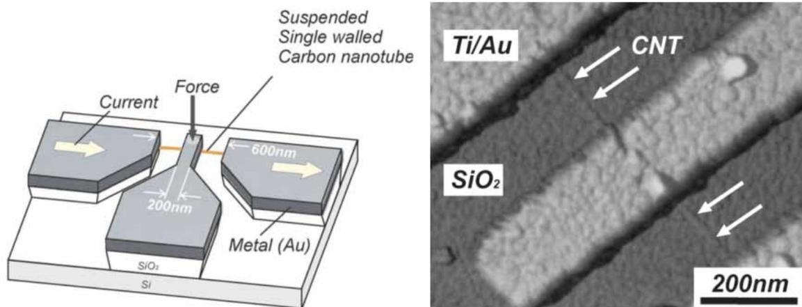
**Figure 6.** Lhs: Schematic illustration of the fabricated CNT-based nanoelectromechanical force sensor. Rhs: AFM image of a contacted SWNT (diameter approximately 1.2 nm). (Reprinted by permission from IEEE: IEEE Sensors Journal [18], © 2006 IEEE)
