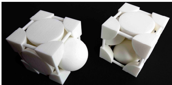
Figure 6: 3D printed opened-up version of the face-centered cubic unit cell with exposed tetrahedral and octahedral interstices (right) and complementary matching piece to “close” the unit cell (left).
