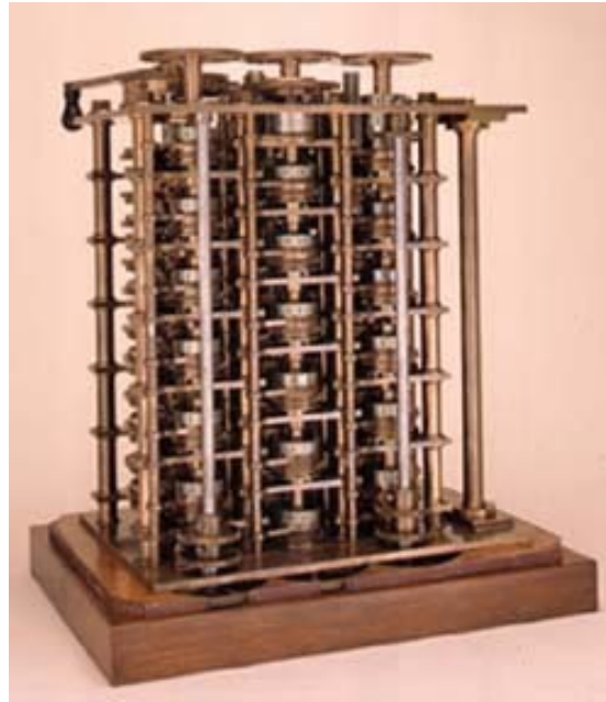
19th century precision engineering Babbage difference engine, 1832
