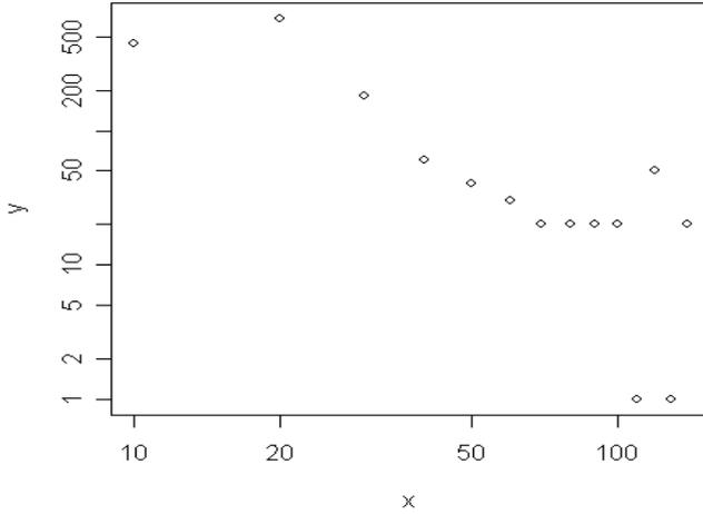
Fig. 4. Distribution of the frequency  $N_p (= y)$  producing excess power  $P_{ex} (= x)$ . To depict log-log curve, values of  $N_p$  and  $P_{ex}$  were arbitrarily multiplied by  $10^3$ . ( $x = 100$  in this figure corresponds to  $P_{ex} = 1$  W)
