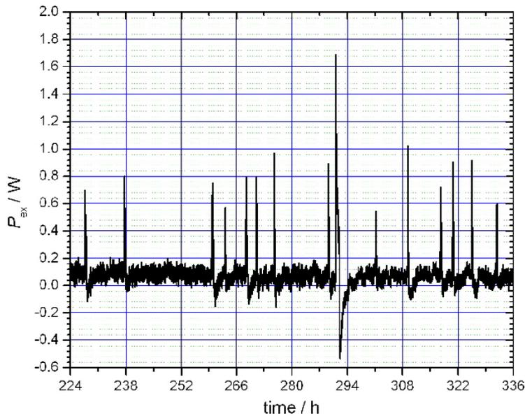
Fig. 2. Excess power pulses and bursts during a 112 hour period of an experiment (061026) which lasted 14 days as a whole.
