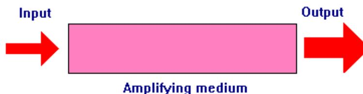
All lasers contain an energized substance that can increase the intensity of light that passes through it. This substance is called the amplifying medium and it can be a solid, a liquid or a gas. The amplifying medium is a rod of yttrium aluminium garnate (YAG) containing neodymium ions. In a dye laser, it is a solution of a fluorescent dye in a solvent such as methanol. In a helium-neon laser, it is a mixture of the gases helium and neon. In a laser
