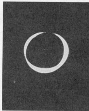
Figure 5.6. (A) An \text{LaB}_6 crystal and the electron distribution when the source is (B) undersaturated and aligned and (C) saturated.
