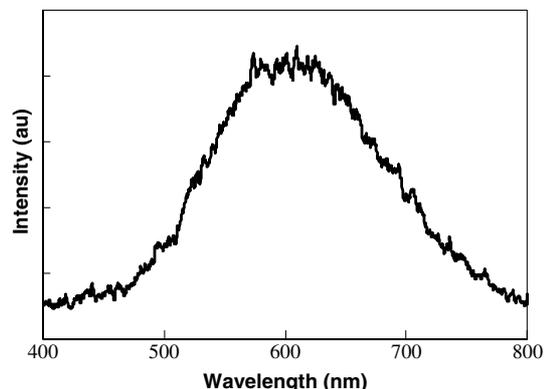
Figure 3. Electroluminescent spectrum of Si nanowires.
