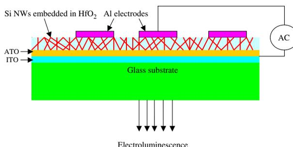
**Figure 1.** Schematic showing cross-sectional view of a Si nanowire electroluminescent device.
