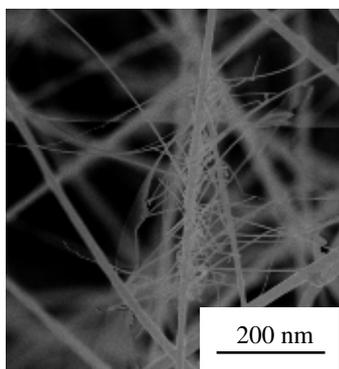
Figure 2. FESEM view of the Si nanowires.
