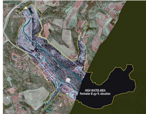
Figure 1. This high-resolution aerial photograph of the Johnstown, Pennsylvania, area is overlaid with the high-water line of former Conemaugh Lake at the time of the catastrophic flood in 1889. Using GIS technology coupled with topographic data, the National Park Service was able to determine the lake's perimeter, calculate the volume of the tremendous flood, and compare the results to historical volume estimates.
