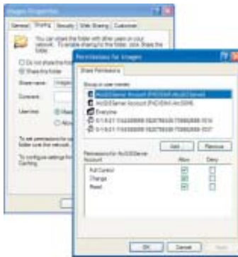
The ArcGIS Server administrator will use operating system tools to manage access to the GIS server and manage privileges on both data and output directories.
