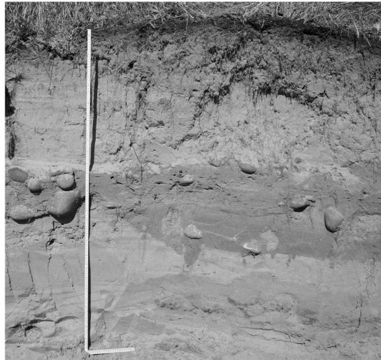
**Figure 11.** Catastrophic flood deposit (dark lithic-rich sand with cobbles) at 60–70 cm depth exposed in spit deposits (light quartz-rich dune sand) in cutbank of Nehalem spit (site CB13) (Figure 8, Table II). Vertical measuring stick scale is 140 cm in length. An optically stimulated luminescence (OSL) sample was collected just below the cobble layer at 100 cm depth (see Figure 13 for full stratigraphic section).
