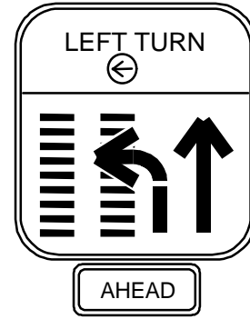
C. Proposed parallel advance warning sign prescribing signal control at grade crossing.
