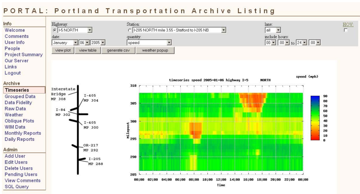
Figure 4: Sample Speed Contour Plot for I-5 North, October 28, 2004
