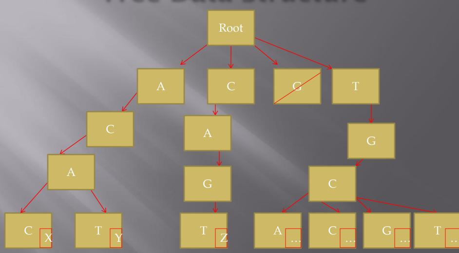
This tree stores: {ACAC, ACAT, CAGT, TGCA, TGCC, TGCG, TGCT} Null pointers are not shown, except for top-most G node. The starting location of the string match is noted in the bottom-most node (e.g. X,Y,Z, etc)
